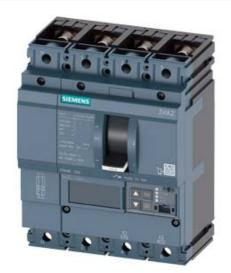
CIRCUIT BREAKER 3VA2 IEC FRAME 250 BREAKING CAPACITY CLASS L ICU=150KA @ 415 V 4POLE, LINE PROTECTION ETU560, LSIG, IN=250A OVERLOAD PROTECTION IR=100A ...250A SHORT CIRCUIT PROTECTION ISD=0,6..10X IN, II=1,5..10X IN NEUTRAL PROTECTION ADJUSTABLE (OFF, UPTO 100%) GROUNDFAULT, SWITCHABLE IG=0,2... 1 X IN, TG=0,050,8MS BUSBAR CONNECTION
