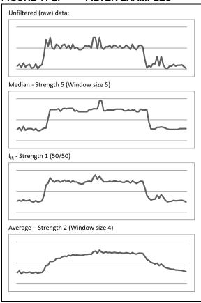
Choosing the correct filtering option for the user's application depends on the environment and sensor. Note that while the median filter has good characteristics, it is not the most efficient and will consume more power than other filters.
