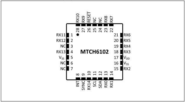
FIGURE 2-2: 28-PIN SSOP
