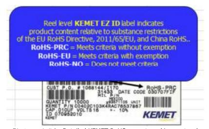
Photograph # 3 - Detailed KEMET RoHS correct marking protocol
