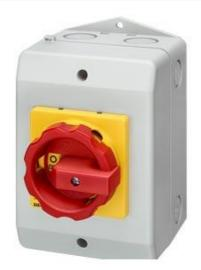
EMERG. STOP SWITCH 4-POLE IU=16, P/AC-23A AT 400V=7.5KW 1 N-TERMINAL + 1 PE-TERMINAL INSULATION-ENCLOSED, IP65 ROTARY ACTUATOR RED/YELLOW (EMERG. STOP)
