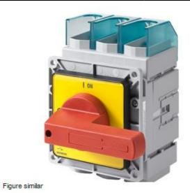
MAIN SWITCH 3-POLE FRONT MOUNTING IU=250A P/AC-23A AT 400V=132KW ROTARY ACTUATOR RED/YELLOW (EMERG. STOP) FOUR-HOLE MOUNTING
