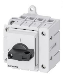
Switch disconnector 3LD3, main switch 3-polig + N, lu 32A operational switch at AC-23 A at 400 V 11,5 kW Distribution board mounting Base mounting with knob-operated mechanism black with auxiliary 1NO+1NC
