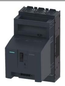
FUSE-SWITCH-DISCONNECTOR 3-POLE, NH00, 160A MOUNTING PLATE CONSTRUCTION COVER LEVEL 45 MM FLAT CONNECTOR FUSE MONITORING ELECTROMECHANICAL
