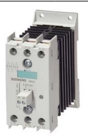
SOLID STATE CONTACTOR 3-P. 3RF2 AC51 10 A 40 DEG. C 48-600 V / 4-30 V DC 3PH.-CONTROLLED SCREW TERMINAL BLOCKING VOLTAGE 1200V
