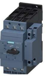
CIRCUIT BREAKER, SIZE S2, FOR MOTOR PROTECTION, CLASS 10, W. OVERLOAD RELAY FUNCTION A-RELEASE 42...52A, N-RELEASE 741A, STANDARD BREAKING CAPACITY
