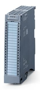
SIPLUS S7-1500 DQ 16x110VDC ST TX RAIL -40 ... +70 Degree C TX with 85 Degree C for 10 min with Conformal Coating BasedOn 6ES7522-5EH00-0AB0 . DQ 16x24 ... 48VUC/125VDC/ 0.5A; 16 Channels in Groups of 1, 0.5A per Group; Substitute Value; Please note Derating
