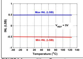
FIGURE 3-3: INL vs. Temperature.
