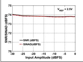
**FIGURE 4-18:** SNR/SINAD vs. Input Amplitude:  $F_{IN} = 10 \text{ kHz}$ .
