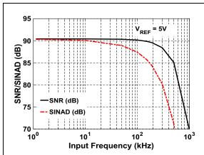
FIGURE 2-19: SNR/SINAD vs.Input Frequency:  $V_{IN} = -1$  dBFS.
