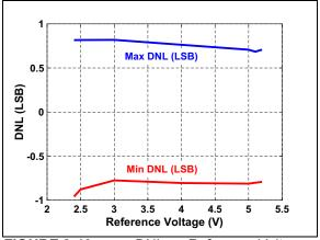
FIGURE 2-10: DNL vs. Reference Voltage.
