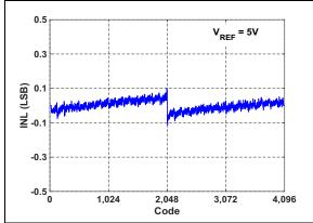
FIGURE 4-1: INL vs. Output Code.
