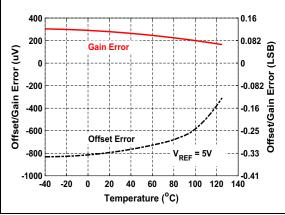
**FIGURE 4-27:** Offset and Gain Error vs. Temperature:  $V_{REF} = 5V$ .
