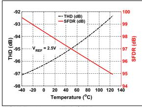
**FIGURE 2-23:** THD/SFDR vs. Temperature:  $V_{RFF} = 2.5V$ .
