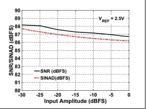
**FIGURE 2-18:** SNR/SINAD vs. Input Amplitude:  $F_{IN} = 10 \text{ kHz}$ .
