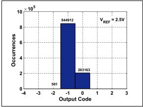
FIGURE 3-29: Shorted Input Histogram:  $V_{REF} = 2.5V$ .
