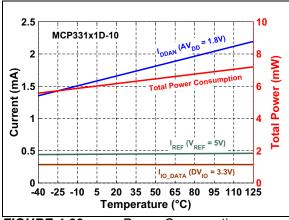
FIGURE 4-33: Power Consumption vs. Temperature:  $C_{LOAD\ SDO} = 20 \text{ pF.}$
