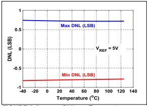
FIGURE 2-6: DNL vs. Temperature.
