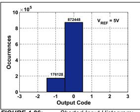
**FIGURE 4-26:** Shorted Input Histogram:  $V_{REF} = 5V$ .
