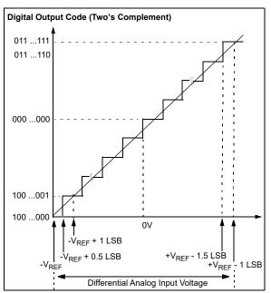
**FIGURE 6-11:** Ideal Transfer Function for Fully-Differential Input Signal.
