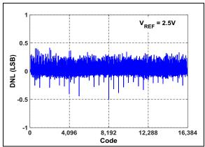
FIGURE 3-5: DNL vs. Output Code.
