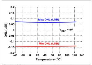
FIGURE 4-6: DNL vs. Temperature.
