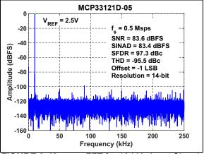
**FIGURE 3-12:** FFT for 10 kHz Input Signal:  $f_{\rm S}$  = 500 kSPS,  $V_{\rm IN}$  = -1 dBFS,  $V_{\rm REF}$  = 2.5V.
