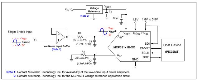
FIGURE 6-7: Pseudo-Differential Unipolar-Input Configuration for Single-Ended Input Signal.
