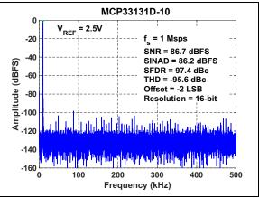
**FIGURE 2-11:** FFT for 10 kHz Input Signal:  $f_S = 1$  Msps,  $V_{IN} = -1$  dBFS,  $V_{REF} = 2.5V$ .
