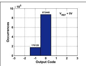
FIGURE 3-26: Shorted Input Histogram: V<sub>RFF</sub> = 5V.
