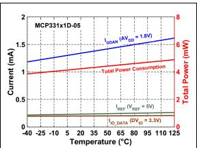
**FIGURE 2-36:** Power Consumption vs. Temperature:  $C_{LOAD}$  SDO = 20 pF.
