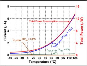
**FIGURE 3-34:** Power Consumption vs. Temperature during Shutdown.
