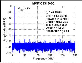
**FIGURE 2-9:** FFT for 10 kHz Input Signal:  $f_S = 500 \text{ kSPS}$ ,  $V_{IN} = -1 \text{ dBFS}$ ,  $V_{REF} = 5V$ .
