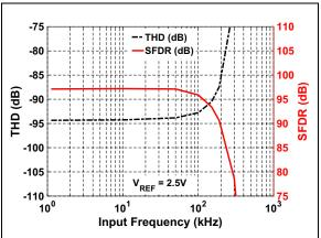
FIGURE 4-24: THD/SFDR vs. Input Frequency: V<sub>REF</sub> = 2.5V.
