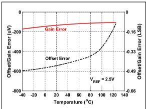
**FIGURE 4-30:** Offset and Gain Error vs. Temperature:  $V_{REF} = 2.5V$ .
