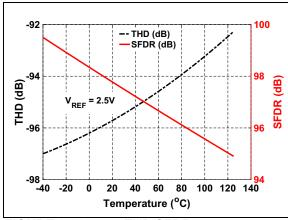
**FIGURE 3-23:** THD/SFDR vs. Temperature:  $V_{RFF} = 2.5V$ .
