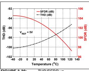
FIGURE 3-20: THD/SFDR vs. Temperature:  $V_{RFF} = 5V$ .
