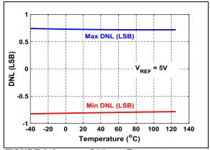
FIGURE 3-6: DNL vs. Temperature.
