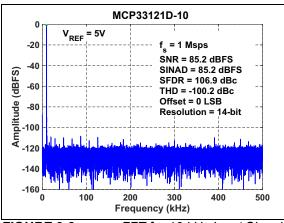
FIGURE 3-8: FFT for 10 kHz Input Signal:  $f_S = 1$  Msps,  $V_{IN} = -1$  dBFS,  $V_{RFF} = 5V$ .
