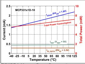
**FIGURE 2-33:** Power Consumption vs. Temperature:  $C_{LOAD\ SDO} = 20 \text{ pF.}$
