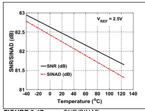
**FIGURE 3-17:** SNR/SINAD vs. Temperature:  $V_{RFF} = 2.5V$ .
