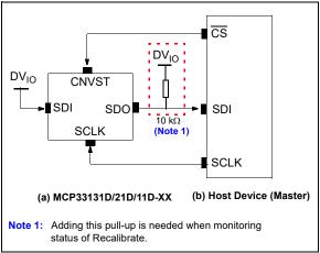
**FIGURE 7-1:** Digital Interface Connection Diagram.
