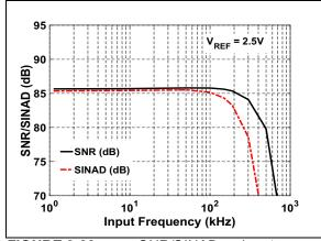
**FIGURE 2-22:** SNR/SINAD vs.Input Frequency:  $V_{IN} = -1$  dBFS.
