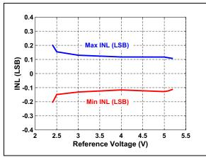
FIGURE 4-7: INL vs. Reference Voltage.
