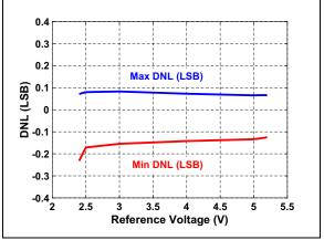
FIGURE 4-10: DNL vs. Reference Voltage.
