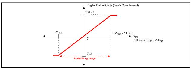
FIGURE 6-3: Transfer Function for Figure 6-7. See the output code example in Table 6-7.
