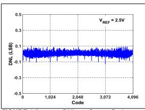
FIGURE 4-2: DNL vs. Output Code.
