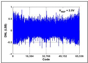
FIGURE 2-5: DNL vs. Output Code.
