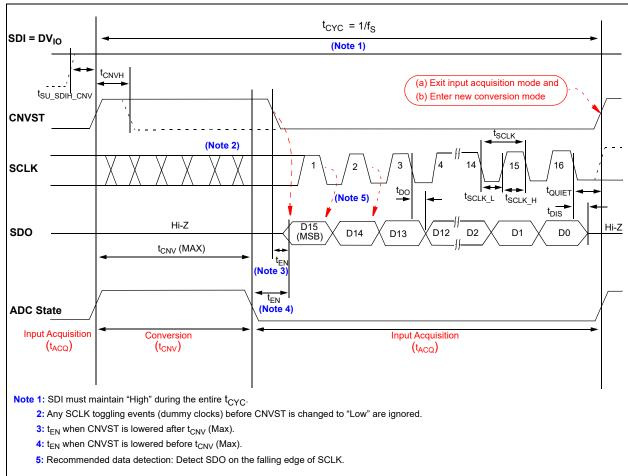
FIGURE 7-2: SPI<sup>TM</sup>Compatible Serial Interface Timing Diagram (16-bit device).
