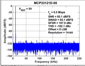
FFT for 10 kHz Input Signal: FIGURE 3-9:  $f_S$  = 500 kSPS,  $V_{IN}$  = -1 dBFS,  $V_{REF}$  = 5V.
