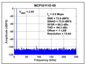
**FIGURE 4-12:** FFT for 10 kHz Input Signal:  $f_S = 500$  kSPS,  $V_{IN} = -1$  dBFS,  $V_{REF} = 2.5V$ .
