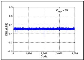
FIGURE 4-5: DNL vs. Output Code.
