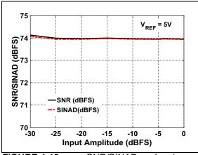
**FIGURE 4-15:** SNR/SINAD vs. Input Amplitude:  $F_{IN} = 10 \text{ kHz}$ .
