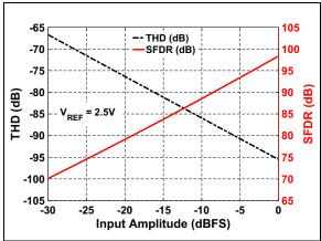
**FIGURE 3-28:** THD/SFDR vs. Input Amplitude:  $V_{RFF} = 2.5V$ .
