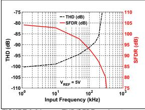
**FIGURE 3-21:** THD/SFDR vs. Input Frequency:  $V_{REF} = 5V$ .
