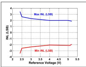
FIGURE 2-7: INL vs. Reference Voltage.
