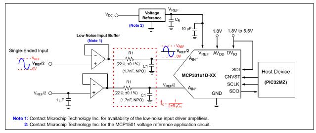
FIGURE 6-5: Pseudo-Differential Bipolar-Input Configuration for Single-Ended Input Signal.
