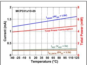
FIGURE 3-36: Power Consumption vs.
