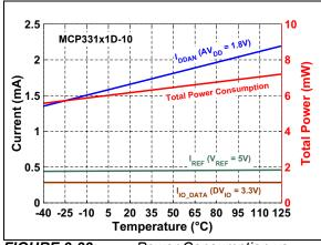
**FIGURE 3-33:** Power Consumption vs. Temperature:  $C_{LOAD\ SDO} = 20 \text{ pF.}$
