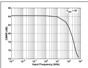
FIGURE 4-31: CMRR vs. Input Frequency: V<sub>RFF</sub> = 5V.
