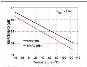
**FIGURE 2-17:** SNR/SINAD vs. Temperature:  $V_{RFF} = 2.5V$ .
