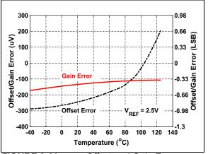
**FIGURE 3-30:** Offset and Gain Error vs. Temperature:  $V_{REF} = 2.5V$ .
