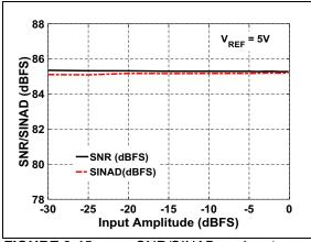
**FIGURE 3-15:** SNR/SINAD vs. Input Amplitude:  $F_{IN}$  = 10 kHz.
