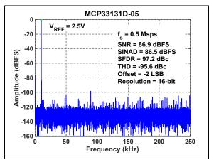
**FIGURE 2-12:** FFT for 10 kHz Input Signal:  $f_S = 500$  kSPS,  $V_{IN} = -1$  dBFS,  $V_{REF} = 2.5V$ .
