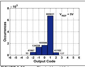
FIGURE 2-26: Shorted Input Histogram: V<sub>RFF</sub> = 5V.
