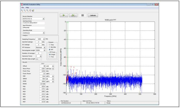
FIGURE 8-2: PC-Based Graphical User Interface Software.
