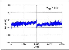
FIGURE 4-4: INL vs. Output Code.
