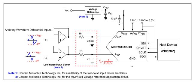
FIGURE 6-4: Input Configuration for Arbitrary Waveform Input Signals.
