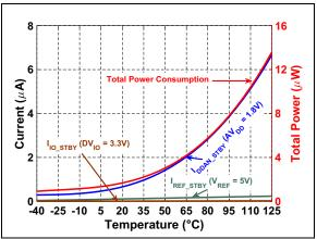
**FIGURE 2-34:** Power Consumption vs. Temperature during Shutdown.
