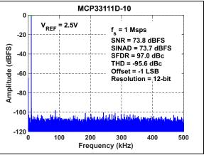
**FIGURE 4-11:** FFT for 10 kHz Input Signal:  $f_S = 1$  Msps,  $V_{IN} = -1$  dBFS,  $V_{REF} = 2.5V$ .
