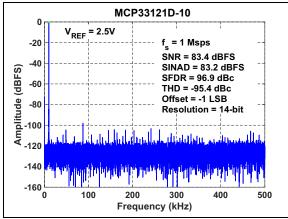
**FIGURE 3-11:** FFT for 10 kHz Input Signal:  $f_S$  = 1 Msps,  $V_{IN}$  = -1 dBFS,  $V_{REF}$  = 2.5V.
