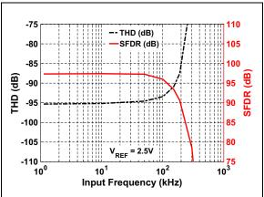
FIGURE 3-24: THD/SFDR vs. Input Frequency: V<sub>REF</sub> = 2.5V.
