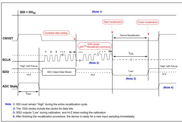
FIGURE 7-3: Recalibrate Command Timing Diagram.
