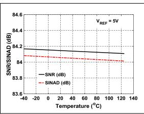
**FIGURE 3-14:** SNR/SINAD vs. Temperature:  $V_{REF} = 5V$ .
