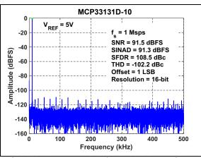
**FIGURE 2-8:** FFT for 10 kHz Input Signal:  $f_S = 1$  Msps,  $V_{IN} = -1$  dBFS,  $V_{REF} = 5V$ .
