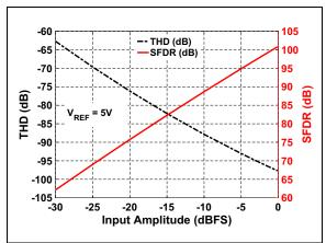
**FIGURE 4-25:** THD/SFDR vs. Input Amplitude:  $V_{RFF} = 5V$ .
