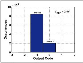
**FIGURE 4-29:** Shorted Input Histogram:  $V_{REF} = 2.5V$ .
