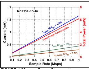
FIGURE 4-32: Power Consumption vs. Sample Rate:  $C_{LOAD\ SDO} = 20 \text{ pF}$ .
