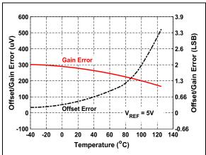
**FIGURE 2-27:** Offset and Gain Error vs. Temperature:  $V_{REF} = 5V$ .
