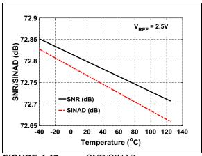
**FIGURE 4-17:** SNR/SINAD vs. Temperature:  $V_{RFF} = 2.5V$ .
