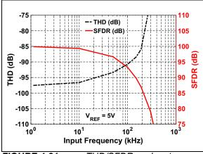
**FIGURE 4-21:** THD/SFDR vs. Input Frequency:  $V_{REF} = 5V$ .
