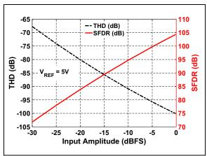
**FIGURE 2-25:** THD/SFDR vs. Input Amplitude:  $V_{RFF} = 5V$ .
