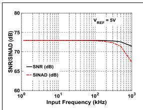
**FIGURE 4-19:** SNR/SINAD vs. Input Frequency:  $V_{IN} = -1$  dBFS
