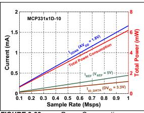
FIGURE 2-32: Power Consumption vs. Sample Rate:  $C_{LOAD\ SDO} = 20 \text{ pF}$ .
