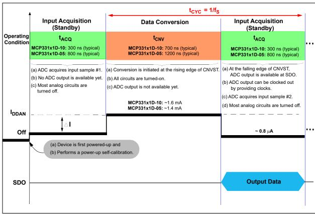
FIGURE 6-10: Device Operating Sequence.
