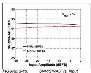
Amplitude:  $F_{IN} = 10 \text{ kHz}$ .
