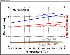
**FIGURE 4-36:** Power Consumption vs. Temperature:  $C_{LOAD}$  SDO = 20 pF.
