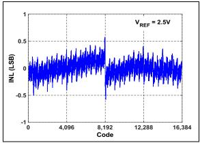
FIGURE 3-4: INL vs. Output Code.
