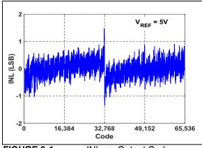
FIGURE 2-1: INL vs. Output Code.
