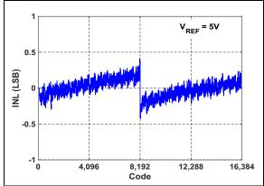
FIGURE 3-1: INL vs. Output Code.
