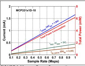
FIGURE 3-32: Power Consumption vs. Sample Rate:  $C_{LOAD\ SDO} = 20 \text{ pF}$ .
