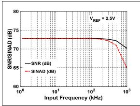
**FIGURE 4-22:** SNR/SINAD vs. Input Frequency:  $V_{IN} = -1$  dBFS.
