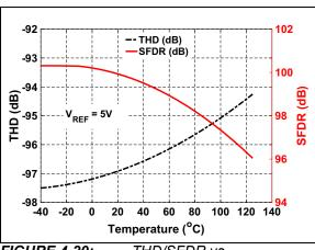
FIGURE 4-20: THD/SFDR vs. Temperature:  $V_{RFF} = 5V$ .
