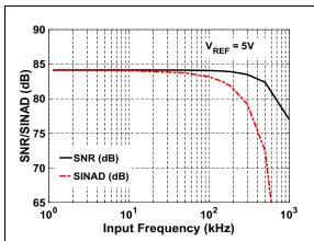
FIGURE 3-19: SNR/SINAD vs.Input Frequency:  $V_{IN} = -1$  dBFS.
