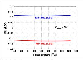
FIGURE 4-3: INL vs. Temperature.
