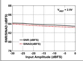
**FIGURE 3-18:** SNR/SINAD vs. Input Amplitude:  $F_{IN} = 10 \text{ kHz}$ .
