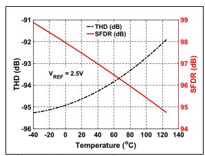
**FIGURE 4-23:** THD/SFDR vs. Temperature:  $V_{RFF} = 2.5V$ .
