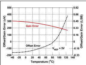
**FIGURE 3-27:** Offset and Gain Error vs. Temperature:  $V_{RFF} = 5V$ .
