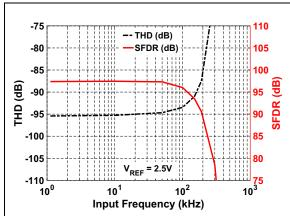
FIGURE 2-24: THD/SFDR vs. Input Frequency: V<sub>REF</sub> = 2.5V.
