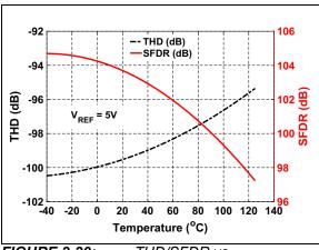
**FIGURE 2-20:** THD/SFDR vs. Temperature:  $V_{RFF} = 5V$ .
