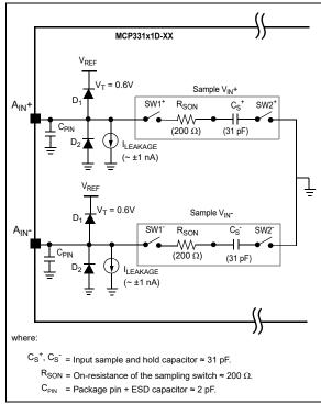
**FIGURE 6-1:** Simplified Equivalent Analog Input Circuit.
