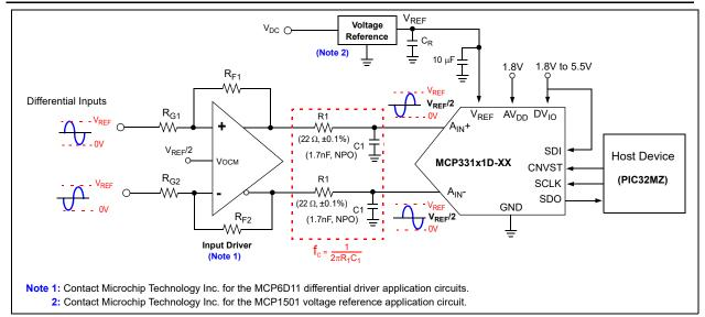
FIGURE 6-2: Input Conditional Circuit for Fully-Differential Input.
