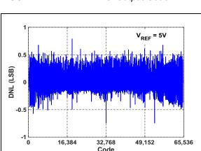
FIGURE 2-2: DNL vs. Output Code.
