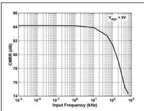
FIGURE 2-31: CMRR vs. Input Frequency: V<sub>RFF</sub> = 5V.
