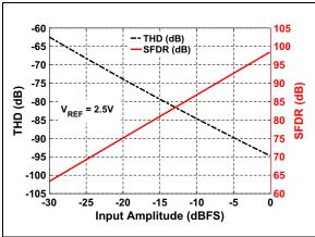
**FIGURE 4-28:** THD/SFDR vs. Input Amplitude:  $V_{REF} = 2.5V$ .
