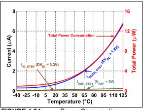
**FIGURE 4-34:** Power Consumption vs. Temperature during Shutdown.
