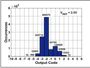
**FIGURE 2-29:** Shorted Input Histogram:  $V_{REF} = 2.5V$ .
