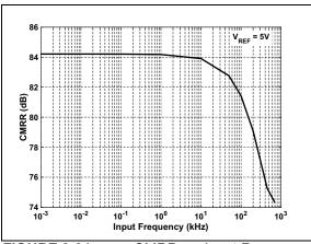
FIGURE 3-31: CMRR vs. Input Frequency: V<sub>RFF</sub> = 5V.
