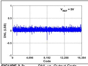
FIGURE 3-2: DNL vs. Output Code.
