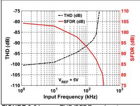
**FIGURE 2-21:** THD/SFDR vs. Input Frequency:  $V_{REF} = 5V$ .
