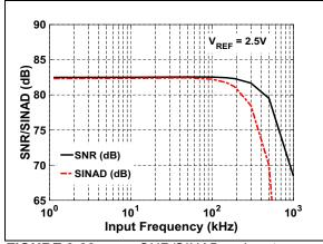
**FIGURE 3-22:** SNR/SINAD vs.Input Frequency:  $V_{IN} = -1$  dBFS.
