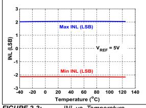
FIGURE 2-3: INL vs. Temperature.
