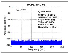
**FIGURE 4-9:** FFT for 10 kHz Input Signal:  $f_S = 500$  kSPS,  $V_{IN} = -1$  dBFS,  $V_{REF} = 5V$ .
