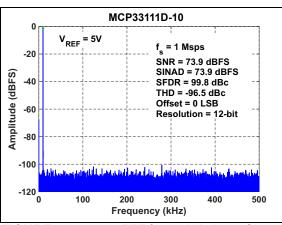
**FIGURE 4-8:** FFT for 10 kHz Input Signal:  $f_S = 1$  Msps,  $V_{IN} = -1$  dBFS,  $V_{REF} = 5V$ .
