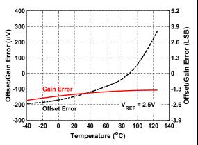
**FIGURE 2-30:** Offset and Gain Error vs. Temperature:  $V_{REF} = 2.5V$ .
