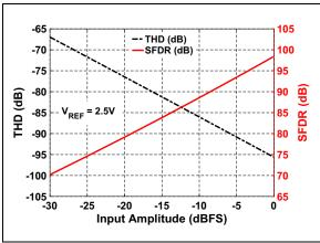
**FIGURE 2-28:** THD/SFDR vs. Input Amplitude:  $V_{REF} = 2.5V$ .
