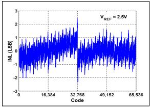
FIGURE 2-4: INL vs. Output Code.
