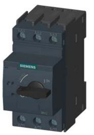
CIRCUIT-BREAKER SZ S00, FOR STARTER COMBINATION, RATED CURRENT 0.8A, N-RELEASE 10 A, SCREW CONNECTION, STANDARD SW. CAPACITY
