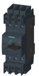
CIRCUIT-BREAKER SZ S00, FOR PLANT PROTECTION, WITH APPROBATION CIRCUIT-BREAKER UL 489. CSA C22.2 NO.5-02. A-RELEASE 0.63 A, N-RELEASE 8.2 A, SCREW CONNECTION, STANDARD SW. CAPACITY
