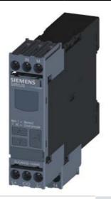
DIGITAL MONITORING RELAY VOLTAGE MONITORING, 22.5MM FOR IO-LINK 10 TO 600V AC/DC OVER- AND UNDERCURRENT HYSTERESIS 0.1 TO 300V ON DELAY TIME TRIPPING DELAY TIME 1 CHANGE-OVER CONTACT, SCREW TERMINAL
