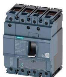
CIRCUIT BREAKER 3VA1 IEC FRAME 160 BREAKING CAPACITY CLASS M ICU=55KA @ 415 V 4-POLE, LINE PROTECTION TM220, ATFM, IN=125A OVERLOAD PROTECTION IR=87,5A ...125A SHORT CIRCUIT PROTECTION II=10 X IN NEUTRAL PROTECTION 50% CABLE CONNECTION
