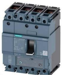
CIRCUIT BREAKER 3VA1 IEC FRAME 160 BREAKING CAPACITY CLASS N ICU=25KA @ 415 V 4-POLE, LINE PROTECTION TM240, ATAM, IN=20A OVERLOAD PROTECTION IR=14A ...20A SHORT CIRCUIT PROTECTION II=5 X IN NEUTRAL PROTECTION 100% BUSBAR CONNECTION
