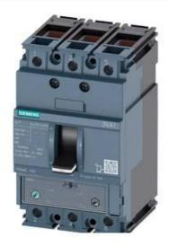
CIRCUIT BREAKER 3VA1 IEC FRAME 160 BREAKING CAPACITY CLASS N ICU=25KA @ 415 V 3-POLE, LINE PROTECTION TM240, ATAM, IN=32A OVERLOAD PROTECTION IR=22,4A ...32A SHORT CIRCUIT PROTECTION II=5...10 X IN CABLE CONNECTION
