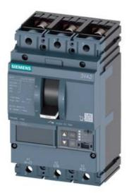
CIRCUIT BREAKER 3VA2 IEC FRAME 160 BREAKING CAPACITY CLASS M ICU=55KA @ 415 V 3POLE, LINE PROTECTION ETU860, LSIG, IN=40A OVERLOAD PROTECTION IR=16A ...40A SHORT CIRCUIT PROTECTION ISD=0,6..10X IN, II=1,5..12X IN NEUTRAL PROTECTION OPTIONAL WITH EXT. CT,UPTO 160% GROUNDFAULT, SWITCHABLE IG=0,2... 1 X IN, TG=0,050,8MS BUSBAR CONNECTION
