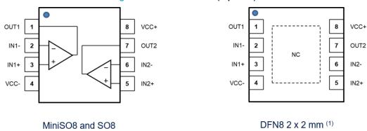
1. The exposed pad of the DFN8 2x2 can be connected to VCC- or left floating.
