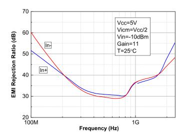
Figure 45. EMIRR on IN+ and IN- pins
