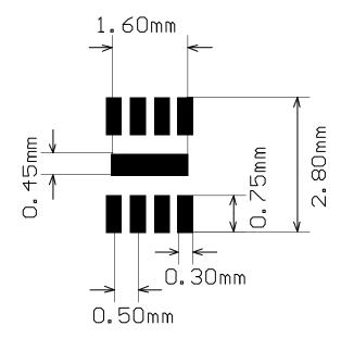
Figure 53. DFN8 2x2 recommended footprint
