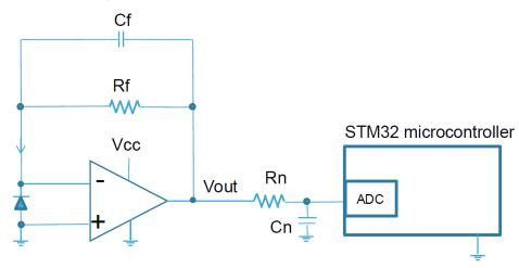
Figure 50. Photodiode transimpedance amplifier circuit
