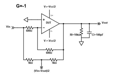
Figure 48. Settling time measurement configuration
