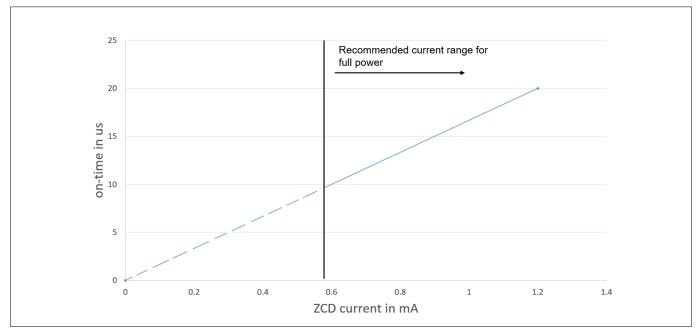
Figure 13 max on-time versus ZCD current
