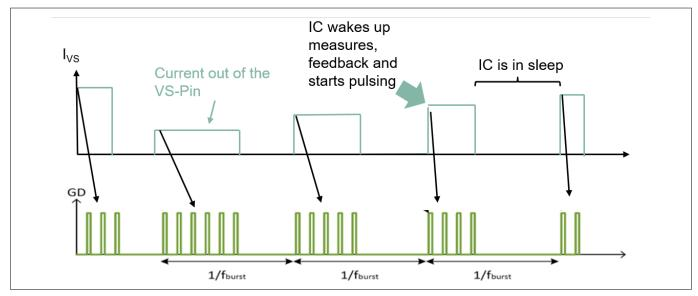
Figure 10 Relation of the feedback current to the duty cycle in the flyback CV topology
