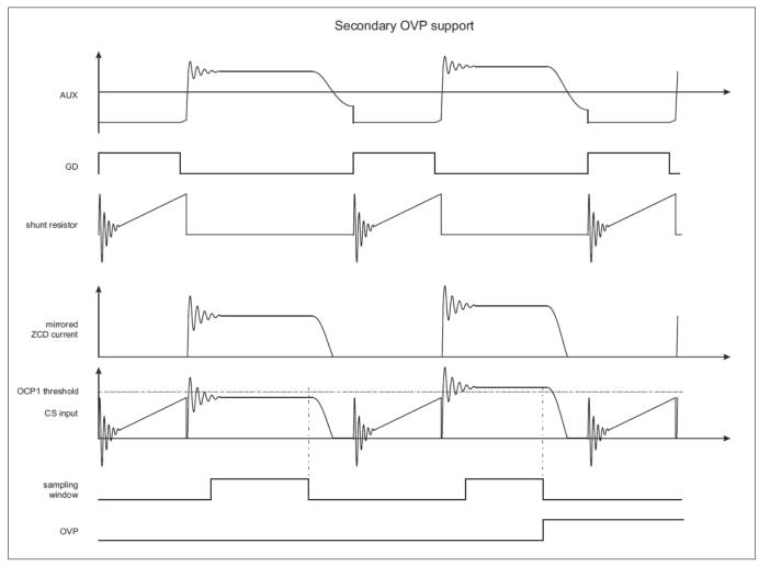
Figure 20 Flyback CS waveform
