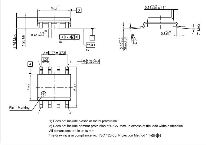
Figure 22 Package dimensions for PG-DSO-8
