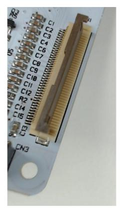
The cable terminal is the same for every screen. With the connector open, slide the cable on the beige part of the connector and gently push it so that it reaches underneath the brown clip. Make sure that the cable is inserted evenly so that when the clip is rotate back into the closed position the two dots shown in the picture are parallel with the connector.
