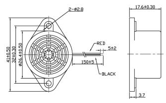
Dimensions : Millimetres Tolerance : ±0.5mm
