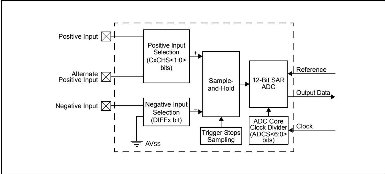
**FIGURE 19-3: SHARED CORE BLOCK DIAGRAM**
