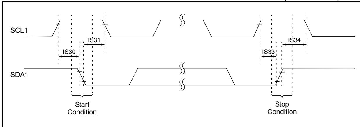
**FIGURE 25-22: I2C1 BUS DATA TIMING CHARACTERISTICS (SLAVE MODE)**
