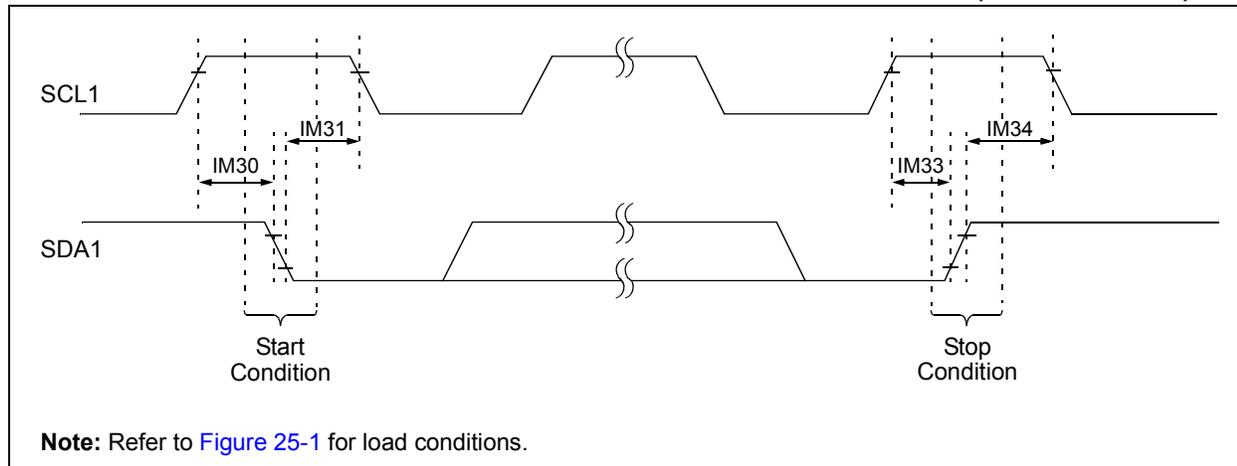
**FIGURE 25-20: I2C1 BUS DATA TIMING CHARACTERISTICS (MASTER MODE)**
