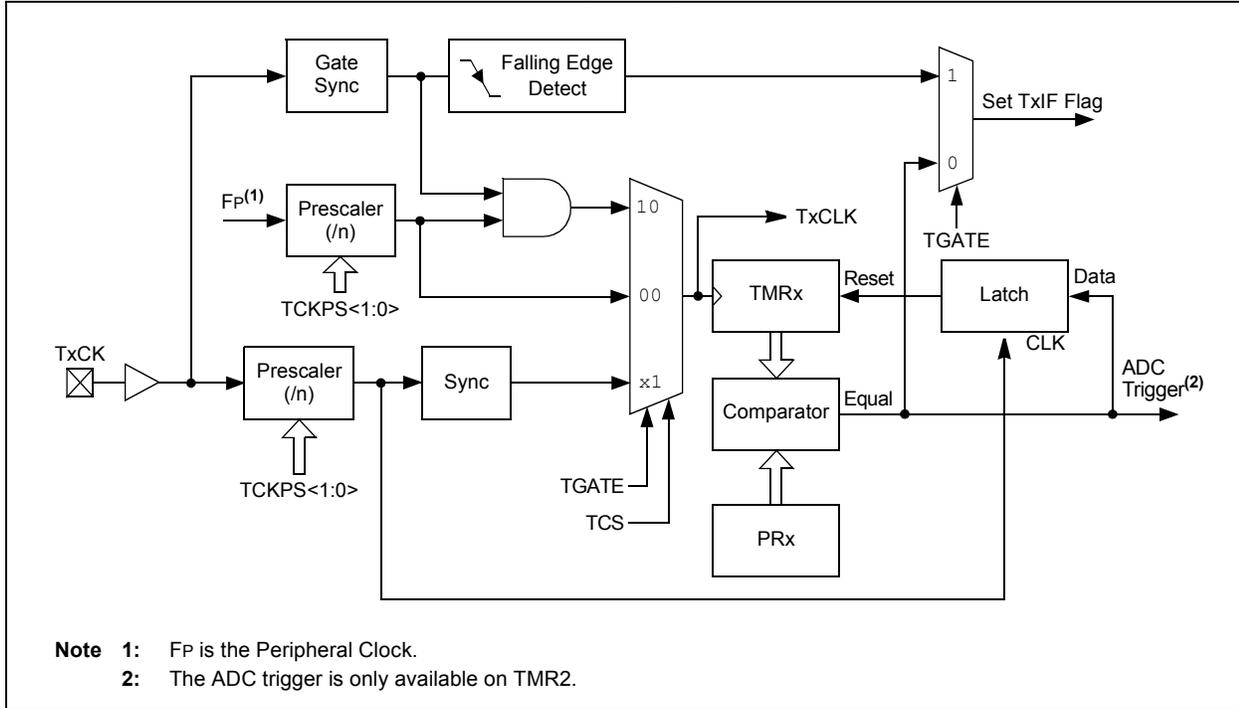
**FIGURE 12-2: TYPE B/TIME C TIMER PAIR BLOCK DIAGRAM (32-BIT TIMER)**
