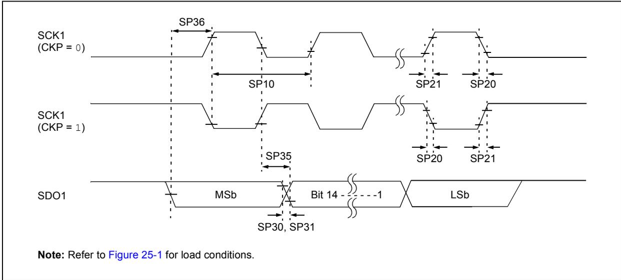
**TABLE 25-32: SPI1 MASTER MODE (HALF-DUPLEX, TRANSMIT ONLY) TIMING REQUIREMENTS**
