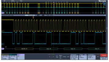
Triggering on a specific address and data packet going across an  $l^2C$  bus. The yellow waveform is clock and the blue waveform is the data. A bus waveform provides decoded packet content including Start, Address, Read/Write, Data, and Stop.
