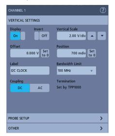
Configuration menus are accessed by simply double-tapping on the item of interest on the display. In this case, the Channel badge was double-tapped to open the channel configuration menu. Menus are dismissed by simply tapping outside of them.
