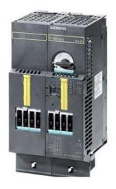
F-RS1E-X FOR ET 200S FAILSAFE REVERSING STARTER SETTING RANGE 2.4...8A, MECHANICAL SWITCHING, ELECTRONIC TROTECTION, AC-3, TO 3KW/400V, CAN BE EXPANDED FOR BRAKE CONTROL MODULE FOR 2DI CONTROL MODUL
