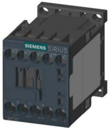
CONTACTOR, AC-3, 7.5KW/400V, 1NC, AC 100V 50HZ, 100...110V 60HZ 3-POLE, SZ S00 SCREW TERMINAL
