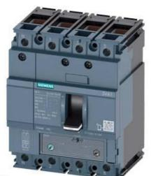
CIRCUIT BREAKER 3VA1 IEC FRAME 160 BREAKING CAPACITY CLASS M ICU=55KA @ 415 V 4-POLE, LINE PROTECTION TM240, ATAM, IN=25A OVERLOAD PROTECTION IR=17,5A ...25A SHORT CIRCUIT PROTECTION II=5...10 X IN NEUTRAL PROTECTION 100% CABLE CONNECTION
