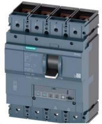
CIRCUIT BREAKER 3VA2 IEC FRAME 400 BREAKING CAPACITY CLASS C ICU=110KA @ 415 V 4-POLE, LINE PROTECTION ETU350, LSI, IN=400A OVERLOAD PROTECTION IR=160A ...400A SHORT CIRCUIT PROTECTION ISD=1,5... 10 X IR, II=10 X IN NEUTRAL PROTECTION ADJUSTABLE(OFF,50%,100%) BUSBAR CONNECTION
