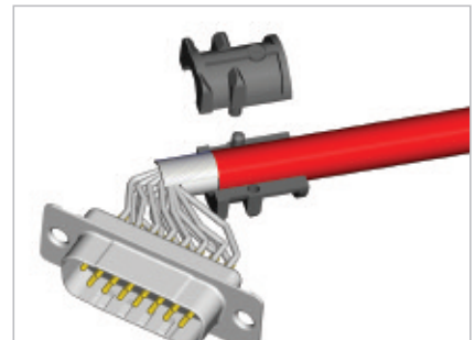
Attach the strain relief around the cable
