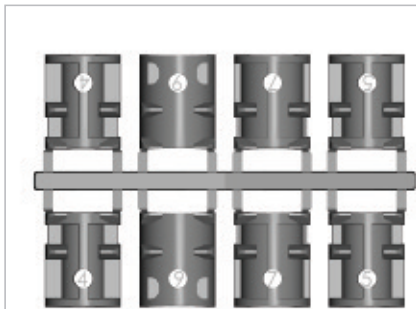
Use two halves of strain relief (different sizes can be mixed)
