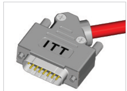
Assemble the other half (screwing force: 100-120 Ncm)
