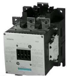
CONTACTOR, 110KW/400V/AC-3 WITHOUT COIL AUXILIARY CONTACTS 2NO+2NC 3-POLE, SIZE S10 BAR CONNECTIONS CONVENT. OPERATING MECHANISM AUX.COND.: SCREW TERMINALS
