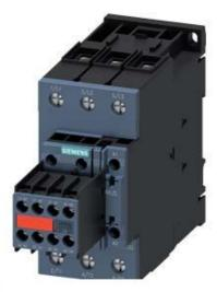
CONTACTOR,AC3:18.5KW/400V, 2NO+2NC, 230V AC 50/60HZ, WITH PLUGGED-IN VARISTOR, 3-POLE, SIZE S2, SCREW TERMINAL, AUXILIARY CONTACT INSEPARABLE
