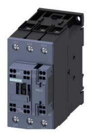
CONTACTOR,AC3:37KW/400V, 1NO+1NC, 110V AC 50HZ, 3-POLE, SIZE S2, SPRING-TYPE TERMINAL
