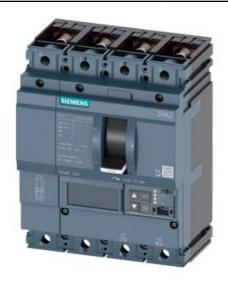
CIRCUIT BREAKER 3VA2 IEC FRAME 250 BREAKING CAPACITY CLASS M ICU=55KA @ 415 V 4POLE, LINE PROTECTION ETU860, LSIG, IN=160A OVERLOAD PROTECTION IR=64A ...160A SHORT CIRCUIT PROTECTION ISD=0,6..10X IN, II=1,5..12X IN NEUTRAL PROTECTION ADJUSTABLE (OFF, UPTO 160%) GROUNDFAULT, SWITCHABLE IG=0,2... 1 X IN, TG=0,050,8MS BUSBAR CONNECTION
