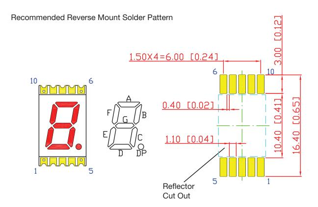
$\label{eq:Dimensions} \mbox{Dimensions in millimeters [inches]} \\ \mbox{Tolerance is $\pm 0.25 mm [.01"] unless otherwise noted}$
