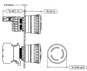
Screw Type Emergency Stop Switches
