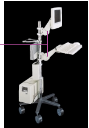
All pivots allow 180° of up/down monitor tilt. Choose a pivot with portrait/landscape (P/L) for 360° monitor rotation and double pivot with P/L for 180° of side-to-side monitor tilt.
