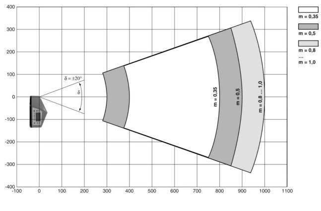
Reading field distance [mm] Reading field height [mm] x y
