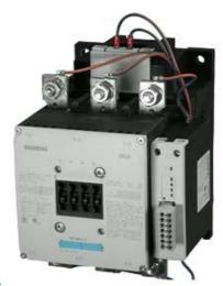
CONTACTOR, 200KW/400V/AC-3 AC(40...60HZ)/DC OPERATION UC 96-127V AUXILIARY CONTACTS 1NO+1NC 3-POLE, SIZE S12 BAR CONNECTIONS ELECTRONIC OPERATING MECHANISM WITH PLC/SIMOCODE INTERFACE AND REMAIN. LIFETIME INDICATOR
