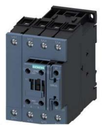
4NO CONTACTOR,AC1:110A 20-33V AC/DC,VARISTOR, 4-POLE, 4NO, SIZE S2, SCREW TERMINAL 1NO+1NC INTEGRATED
