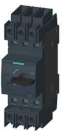
CIRCUIT-BREAKER SZ S00, FOR TRANSFORMER PROTECTION, WITH APPROBATION CIRCUIT-BREAKER UL 489. CSA C22.2 NO.5-02. A-RELEASE 8 A, N-RELEASE 163 A, SCREW CONNECTION, STANDARD SW. CAPACITY
