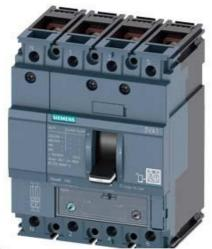
CIRCUIT BREAKER 3VA1 IEC FRAME 160 BREAKING CAPACITY CLASS H ICU=70KA @ 415 V 4-POLE, LINE PROTECTION TM240, ATAM, IN=125A OVERLOAD PROTECTION IR=87,5A ...125A SHORT CIRCUIT PROTECTION II=5...10 X IN NEUTRAL PROTECTION 100% BUSBAR CONNECTION
