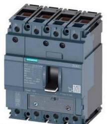
CIRCUIT BREAKER 3VA1 IEC FRAME 160 BREAKING CAPACITY CLASS H ICU=70KA @ 415 V 4-POLE, LINE PROTECTION TM240, ATAM, IN=50A OVERLOAD PROTECTION IR=35A ...50A SHORT CIRCUIT PROTECTION II=5...10 X IN NEUTRAL UNPROTECTED CABLE CONNECTION
