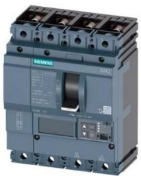
CIRCUIT BREAKER 3VA2 IEC FRAME 100 BREAKING CAPACITY CLASS M ICU=55KA @ 415 V 4POLE, LINE PROTECTION ETU850, LSI, IN=25A OVERLOAD PROTECTION IR=10A ...25A SHORT CIRCUIT PROTECTION ISD=0,6..10X IN, II=1,5..12X IN NEUTRAL PROTECTION ADJUSTABLE (OFF, UPTO 160%) BUSBAR CONNECTION
