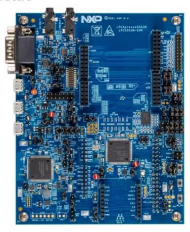
The LPC5536-EVK development board provides the ideal platform for evaluation of and development with the LPC553x MCU based on the Arm® Cortex®-M33 architecture. The board includes a high-performance onboard debug probe and accelerometer, with several options for adding off-the-shelf add-on boards for networking, sensors, displays, and other interfaces.
