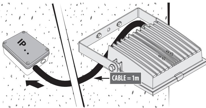
**GB** WARNING: make sure that the connection is made with components that guarantee the IP rating.
