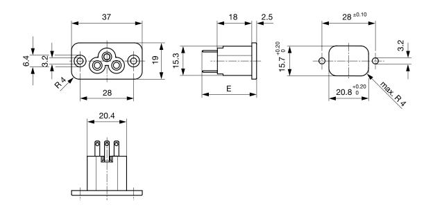
E: Solder terminals short: 19.9 mm E: Solder terminals long: 25.9 mm
