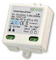
The Tiger Power range of LED drivers are highly reliable and meet latest safety and energy efficiency legislation. The TGR-12V-6W-B provides a 12vdc constant voltage output at up to 500mA (6W) suitable for a wide range of applications including LED strip lighting.
