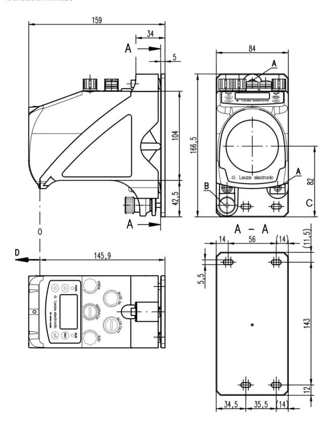
A M 5 screw for alignment
