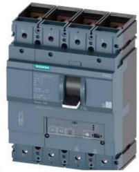
CIRCUIT BREAKER 3VA2 IEC FRAME 630 BREAKING CAPACITY CLASS H ICU=85KA @ 415 V 4-POLE, LINE PROTECTION ETU320, LI, IN=400A OVERLOAD PROTECTION IR=160A ...400A SHORT CIRCUIT PROTECTION II=12 X IN NEUTRAL PROTECTION ADJUSTABLE(OFF,50%,100%) BUSBAR CONNECTION
