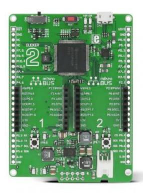
Clicker 2 for MSP432 is a compact development board with two mikroBUS™ sockets for click board connectivity. It carries the SimpleLink™ MSP432™ - ARM® 32-Bit Cortex®-M4F CPU with integrated 1Msps 14-bit SAR-based ADC from Texas Instruments.
